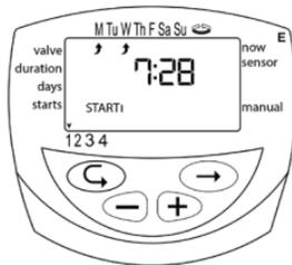
5. To cancel a specific start time, select it by pressing "Enter" (↻) and press "Set" (→). The hour digits will blink. Press "Plus" (+) or "Minus" (-) until the word "OFF" appears on the display.
